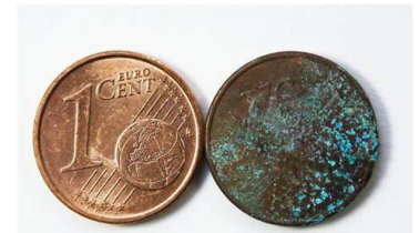
Figure 1. Corroded Copper Coin
