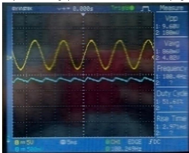
Figure 9-14: LM2907 output without polarised capacitor
