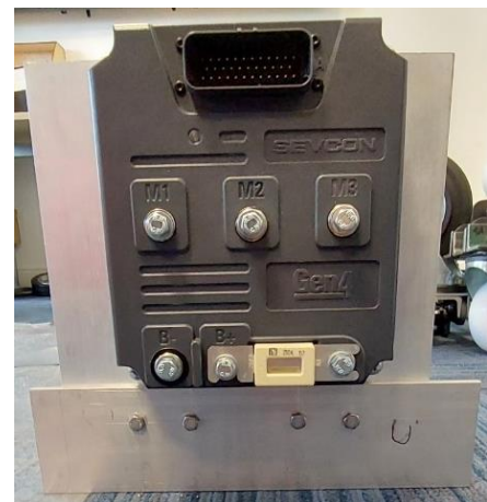
Figure 7.16 – Manufactured Sevcon mount
