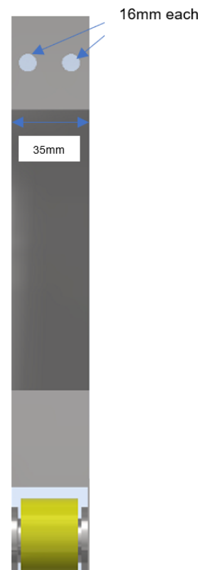
Figure 5-48: Dimensioned Sketch of TC.
